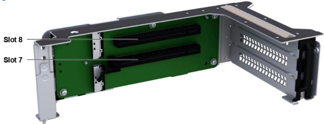
→ [Figure 5-9](#) shows an RC5305L2C riser card installed in I/O module 3.
