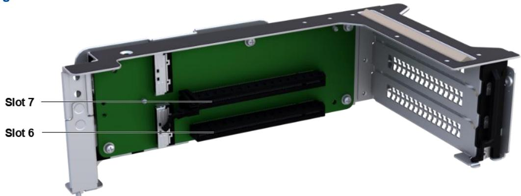
→ [Figure 5-8](#) shows an RC5305L2B riser card installed in I/O module 3.
