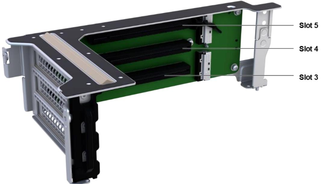
→ [Figure 5-4](#) shows an RC5305R2A riser card installed in I/O module 2.
